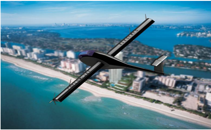
High lift from CFJ would enable aircraft to have a small wing that is more efficient in cruise. Credit: Gecheng Zha/University of Miami
